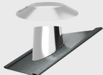
**Roof flashing with lead** : If you want to lead your stainless steel chimney through a roof, you need a suitable roof flashing. Please note that you must also attach a storm collar to the length element above the roof duct to prevent rain or snow from entering the gap.
