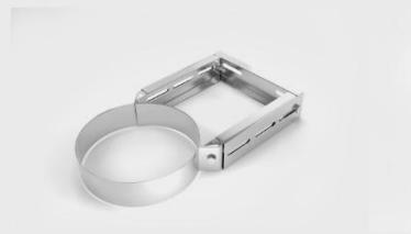
**Adjustable Wall bracket** : The stainless steel wall bracket is used to attach the chimney to the wall. It should be noted that the stainless steel chimney is to be attached to the wall at a distance of 4m by means of wall brackets. In addition, the chimney may stand freely for a maximum of 3m from the last wall bracket. Wall brackets can be connected with wall bracket extensions to allow a larger wall distance.
